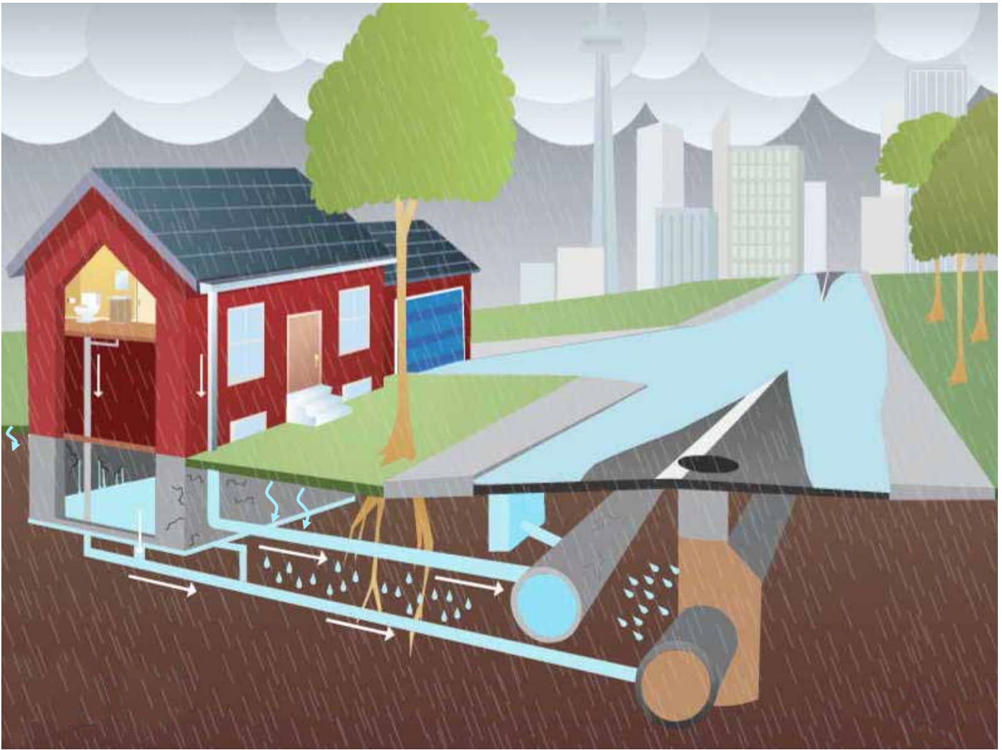
Home drainage and causes of basement flooding, Toronto Water, n.d.
