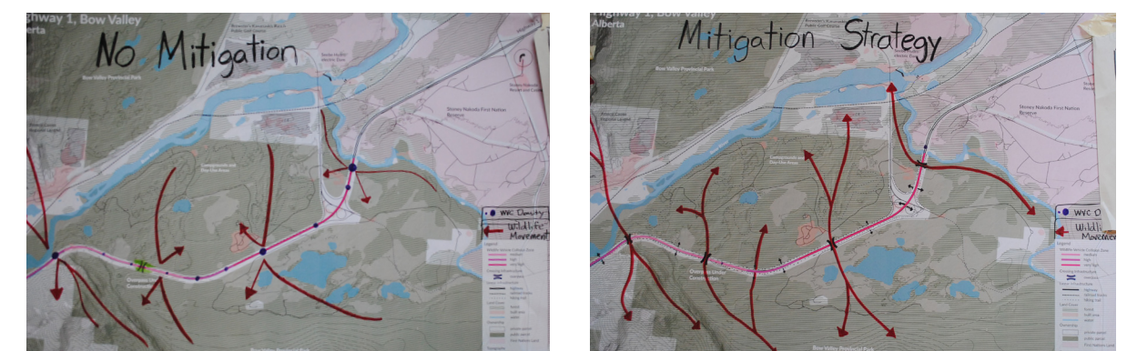
Figure 6 - Visualizations showing the barrier effect of the highway and the benefits to wildlife when mitigation measures are in place can work to communicate the value of crossing infrastructure.
